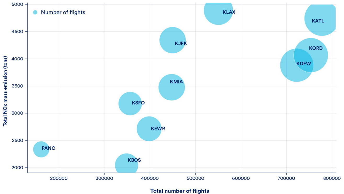
Figure 23: NO x emissions plotted as a function of total flight activity for U.S. airports
