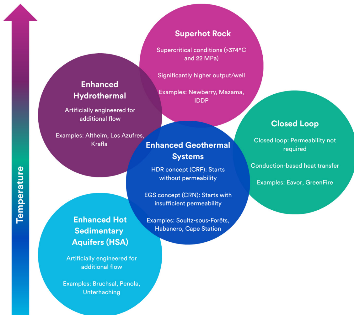
Figure II.2: Blurred Lines Between Geothermal Project Categories EGS (enhanced geothermal system), CRF (crystalline rock with dominant artificial fractures), CRN (crystalline rock with dominant natural fractures or faults). Adapted from (Bloomberg NEF, 2023 and this research).
