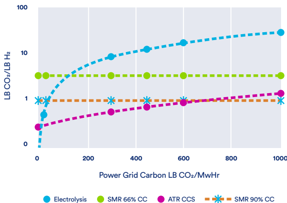
Figure 4: Carbon Emissions – Electrolysis vs ATR CCS vs SMR CCS Carbon Intensity per Lb H 2
