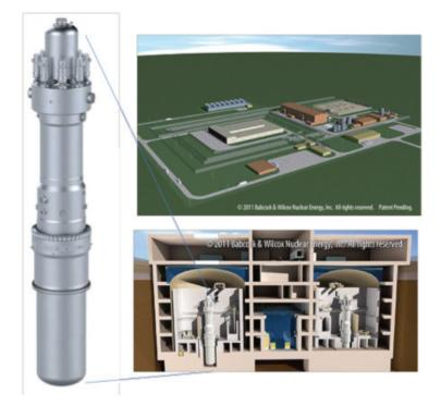
FIGURE 2 Illustrates the mPower 360 MWe Reference Plant with 2 Modules, Below Grade Containment Details and Integral Pressure Vessel FIGURE 3 Illustrates the Reference Westinghouse 225 MWe SMR Plant with one module, Details of the Below Grade Containment and Integral Pressure Vessel
