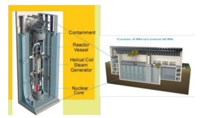
generators, pressurizer and pumps (if part of the design), are housed in a single pressure vessel. The original integral PWR was designed to power the German commercial ship, N.S. Otto Hahn, commissioned in 1968, which sailed without incident for over one million kilometers. The ship was converted to conventional power in 1979 for economic reasons.
