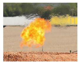
**the gas.** Beyond wasting natural gas, flaring produces numerous pollutants, such as carbon dioxide, NO<sub>x</sub>, and harmful, toxic products of incomplete combustion such as black carbon.
