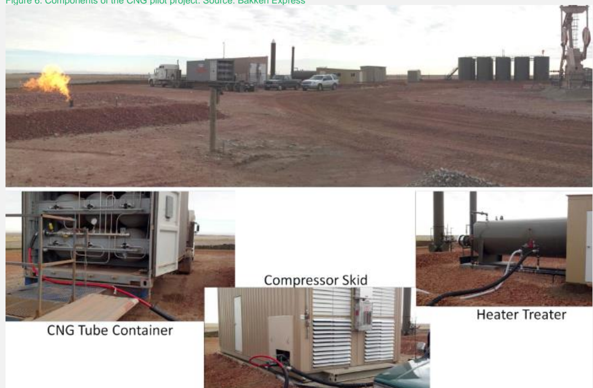
Figure 6: Components of the CNG pilot project. Source: Bakken Express
