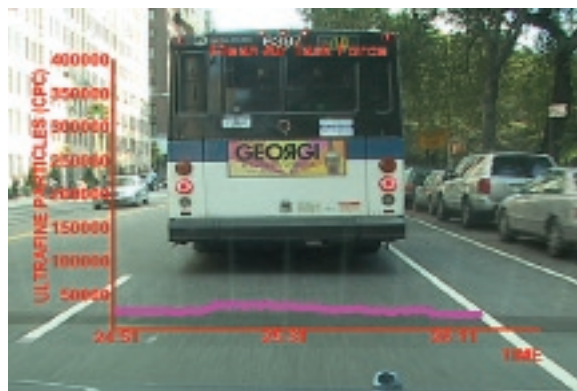
Left: Exhaust from a conventional New York City transit bus infiltrates a car following behind. Right: Ultrafine particle levels behind a bus equipped with a diesel particulate filter are virtually eliminated. To view videos, go to www.catf.us/goto/noescape/
