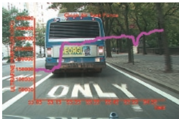
Left: Exhaust from a conventional New York City transit bus infiltrates a car following behind. Right: Ultrafine particle levels behind a bus equipped with a diesel particulate filter are virtually eliminated. To view videos, go to www.catf.us/goto/noescape/
