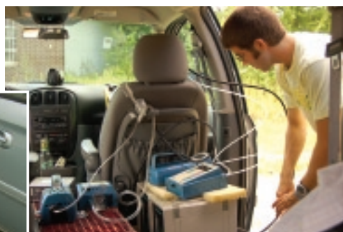
Above: CATF researcher setting up particle monitoring equipment to monitor both cabin and outdoor air simultaneously with two sets of equipment.
