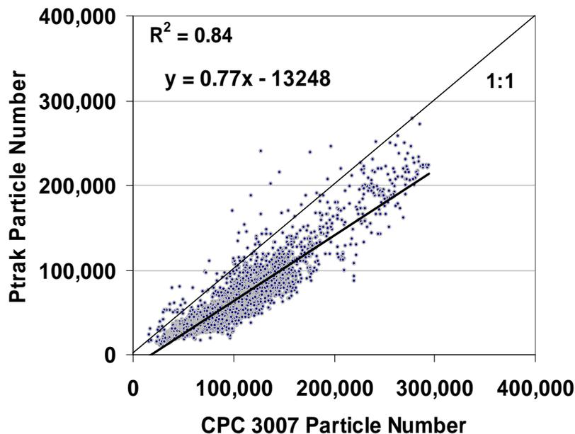
**Above: one of three linear regressions comparing *uncorrected* CPC 3007 to PTrak response. Note that the PTrak underestimates particle count and therefore data in this paper likely represent conservative estimates of ultrafine particle/nanoparticle exposure Black Carbon**
