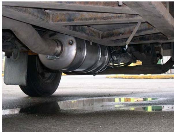
**Above: A catalyzed diesel particulate filter (DPF) is nearly as simple as replacing the muffler. Verification tests by EPA and CARB suggest that DPFs are extremely effective and remove over 85 percent of diesel exhaust particles. Our results confirm that they work in traffic. These filters can typically be installed on vehicles 1994 and newer that have electronic engine systems. Some newer DPFs may be able to be used on all engines.**
