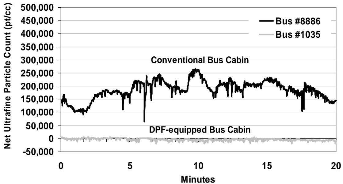
**Above: Comparison of cabin air in conventional Boston transit bus (black line) with a retrofit bus (blue line). (Note this represents the most polluted conventional bus we rode vs the cleanest DPF equipped bus.)**
