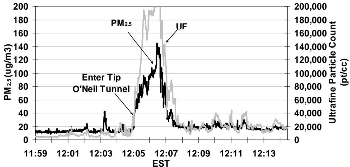
Above: Single pass through Boston motor vehicle tunnel demonstrates dramatic increases in fine and ultrafine particles in the monitoring vehicle (window partially open.)
