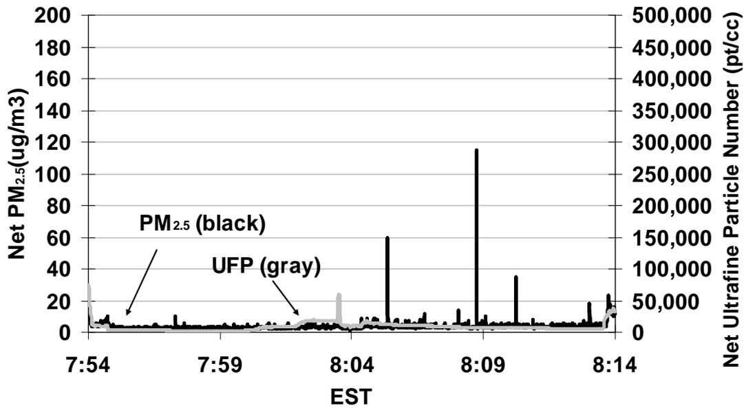
Above: Push train from Lincoln to Porter Square in Boston MBTA in contrast to pull train shows little to no buildup of UFPs and  $PM_{2.5}$ .
