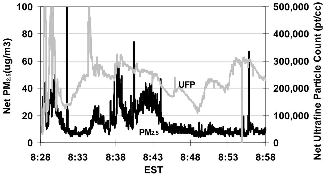
Above: Pull train returning from Porter Square to Lincoln in Boston MBTA shows substantial buildup of UFPs and PM<sub>2.5</sub>.
