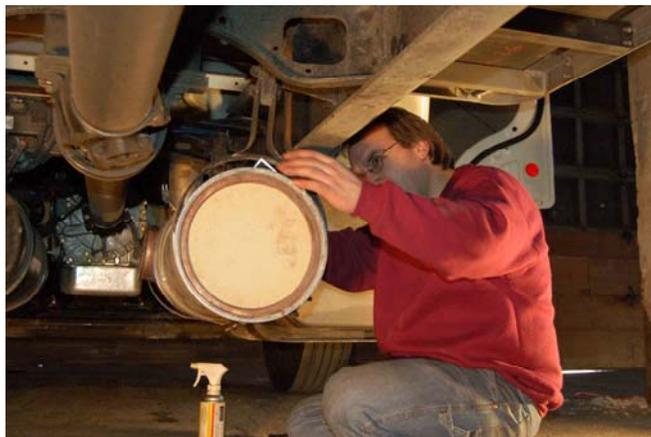
**Above: the box truck was retrofitted in short order. Note the internal DPF's honeycomb trap facing the viewer.**
