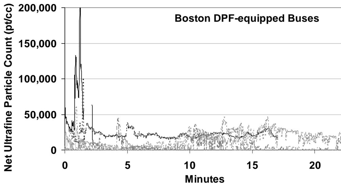
Above: Comparative net ultrafine particle exposures in conventional and DPF-equipped transit buses in Boston. Exposures were found to be lower on DPF equipped buses. This finding is consistent with CATF's school bus study results (<http://www.catf.us/publications/view/82> )
