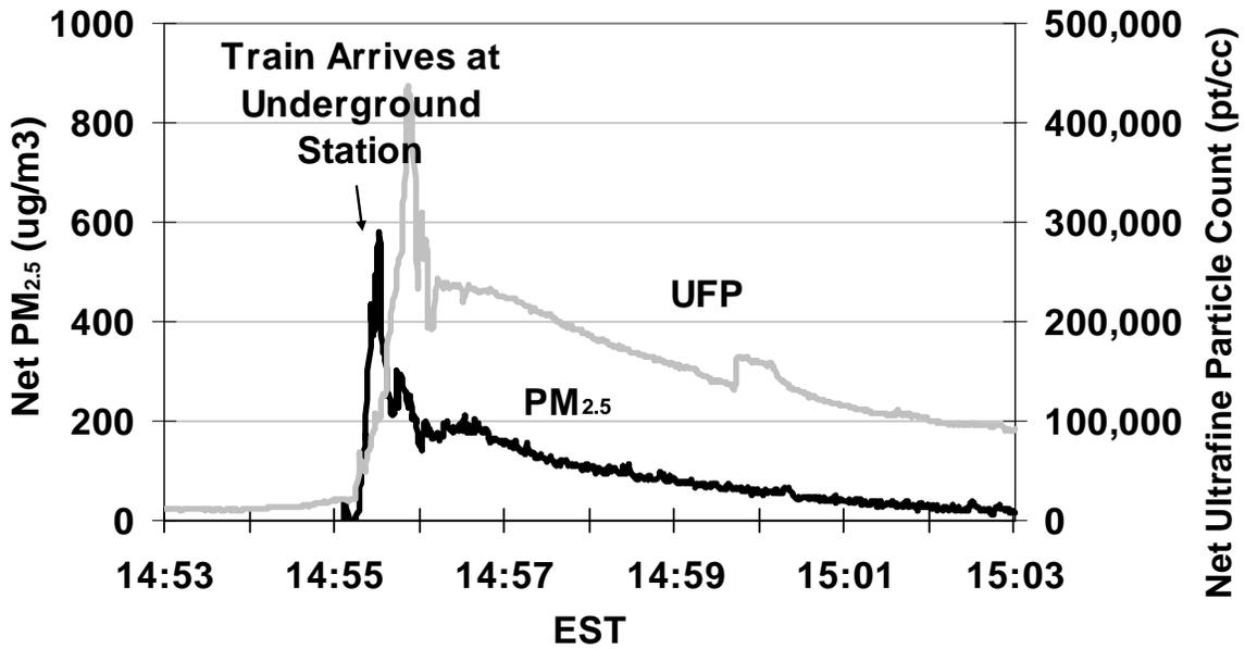
Above: Plot shows impact of underground station on coach air quality on “push” train. Exposures from the underground station decay but generally persist through much of the rest of the train ride
