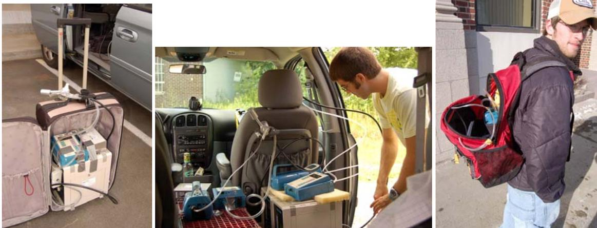
**Left: roll-around monitoring in portable luggage. Center: CATF researcher setting up particle monitoring equipment to monitor both cabin and outdoor air simultaneously with 2 sets of equipment. Right: Backpack monitoring.**
