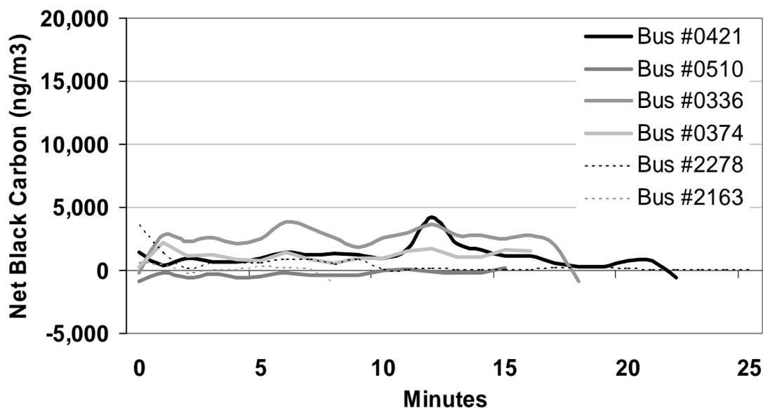
Above: Boston's DPF-Equipped and CNG buses (that are not influenced by other diesels in the roadway) were characterized by low in-cabin black carbon levels.
