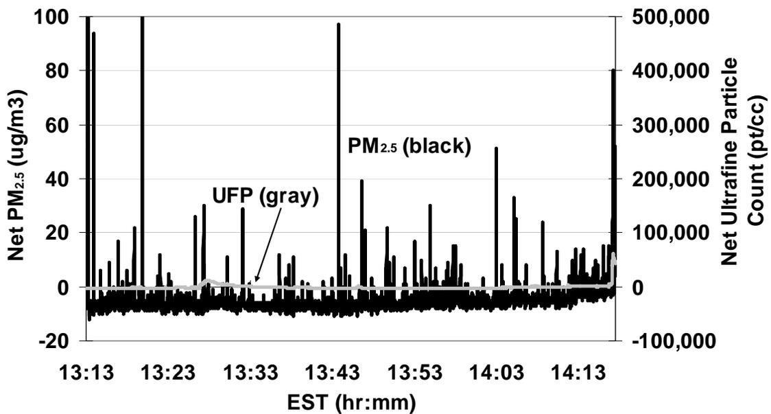
Above: “Push” train exposure signature in New York City commuter rail run with very low net exposures to ultrafine particles and PM<sub>2.5</sub>.
