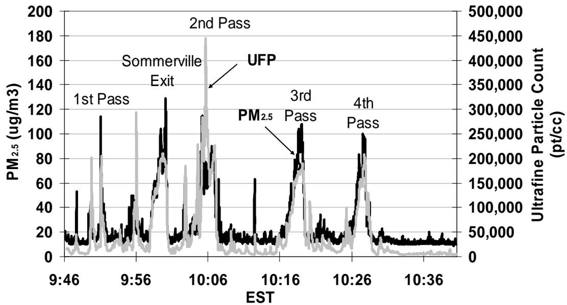
Above: Multiple passes through Boston’s “Big Dig” Thomas P. O’Neill tunnel document high levels of all four measured pollutants inside the tunnels. Exposures were reduced somewhat with windows closed, but substantially reduced when internal recirculation was used in the monitoring vehicle as determined in a 2 car parallel / simultaneous run experiment in the tunnels.
