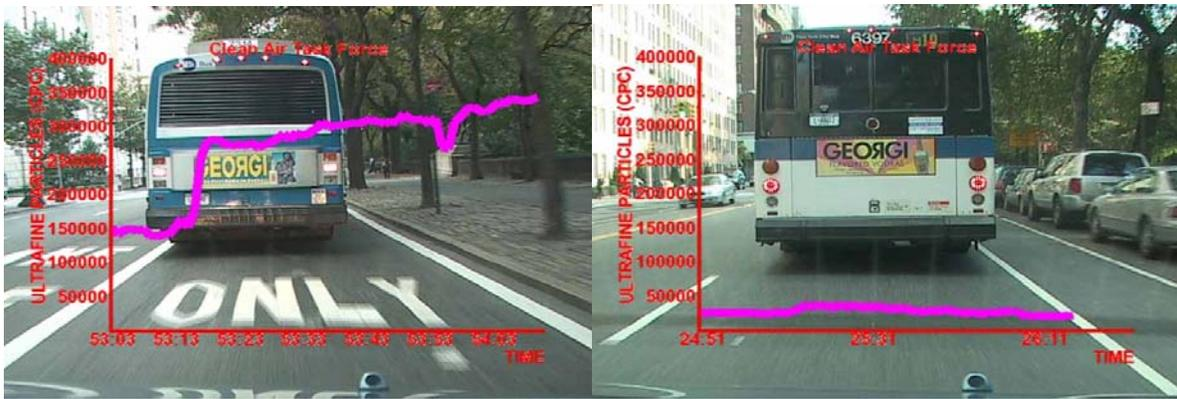
**New York City bus chase proves DPFs Work. *Left:* Real-time measurements documents tailpipe plume polluting chase vehicle following a New York MTA bus without a diesel particulate filter (DPF). *Right:* A NYC Transit bus equipped with a DPF eliminates the soot plume behind the bus. (For video see [www.catf.us/goto/noescape/](http://www.catf.us/goto/noescape/) )**
