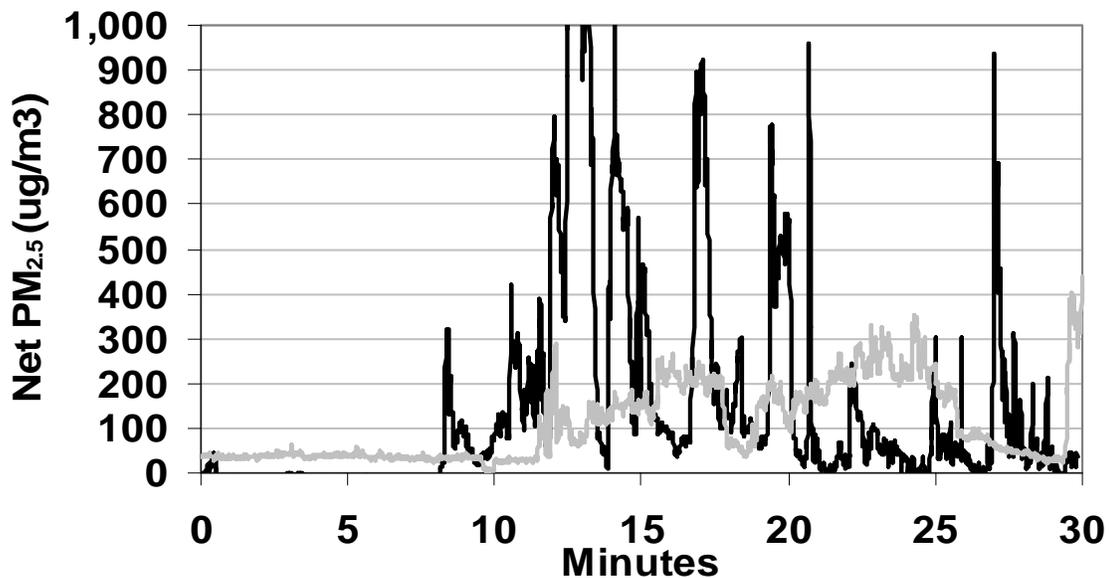
**High Net  $PM_{2.5}$  exposures on 2 Boston Harbor ferry runs. Exhaust smoke eddies behind the boat and enters through the rear door.**
