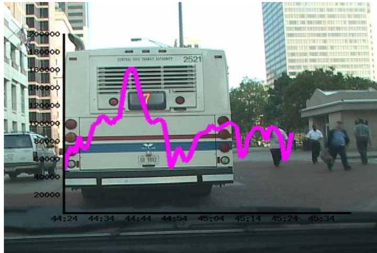
**Above: Columbus biodiesel bus leaves ultrafine particle pollution in its wake as detected in CATF chase vehicle.**
