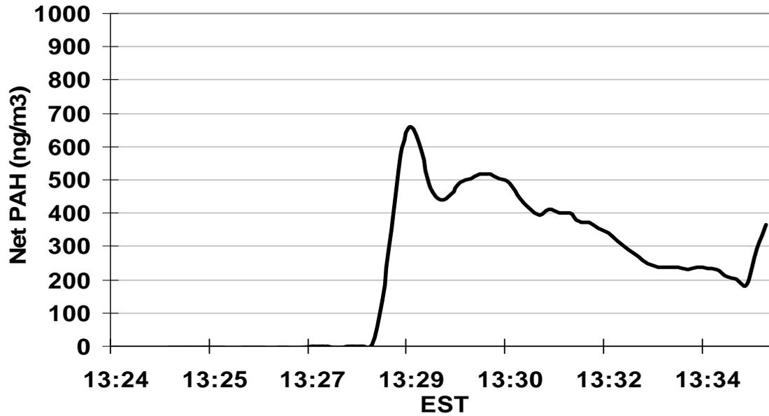
Boston train with locomotive in rear is polluted by particulate PAH when entering the underground Back Bay station at 13:28. Note parallel curve to UFP and PM<sub>2.5</sub> plots above.
