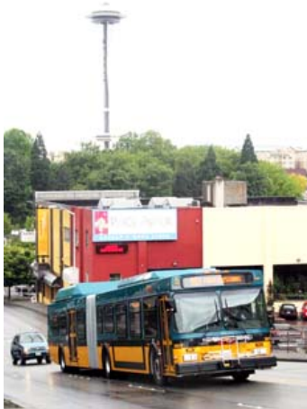
Seattle diesel-electric hybrid bus (courtesy, New Flyer)
