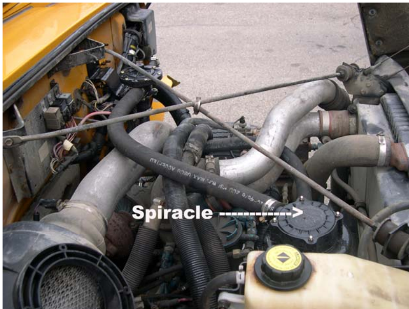
A crankcase ventilation filtration system, the Donaldson Spiracle (black canisters connected by black hose on top of engine) reroutes crankcase emissions through the exhaust system and emissions controls.
