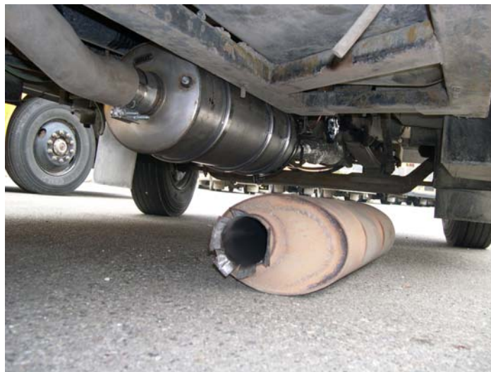
Installation of a DPF requires replacement of the muffler and tailpipe.
