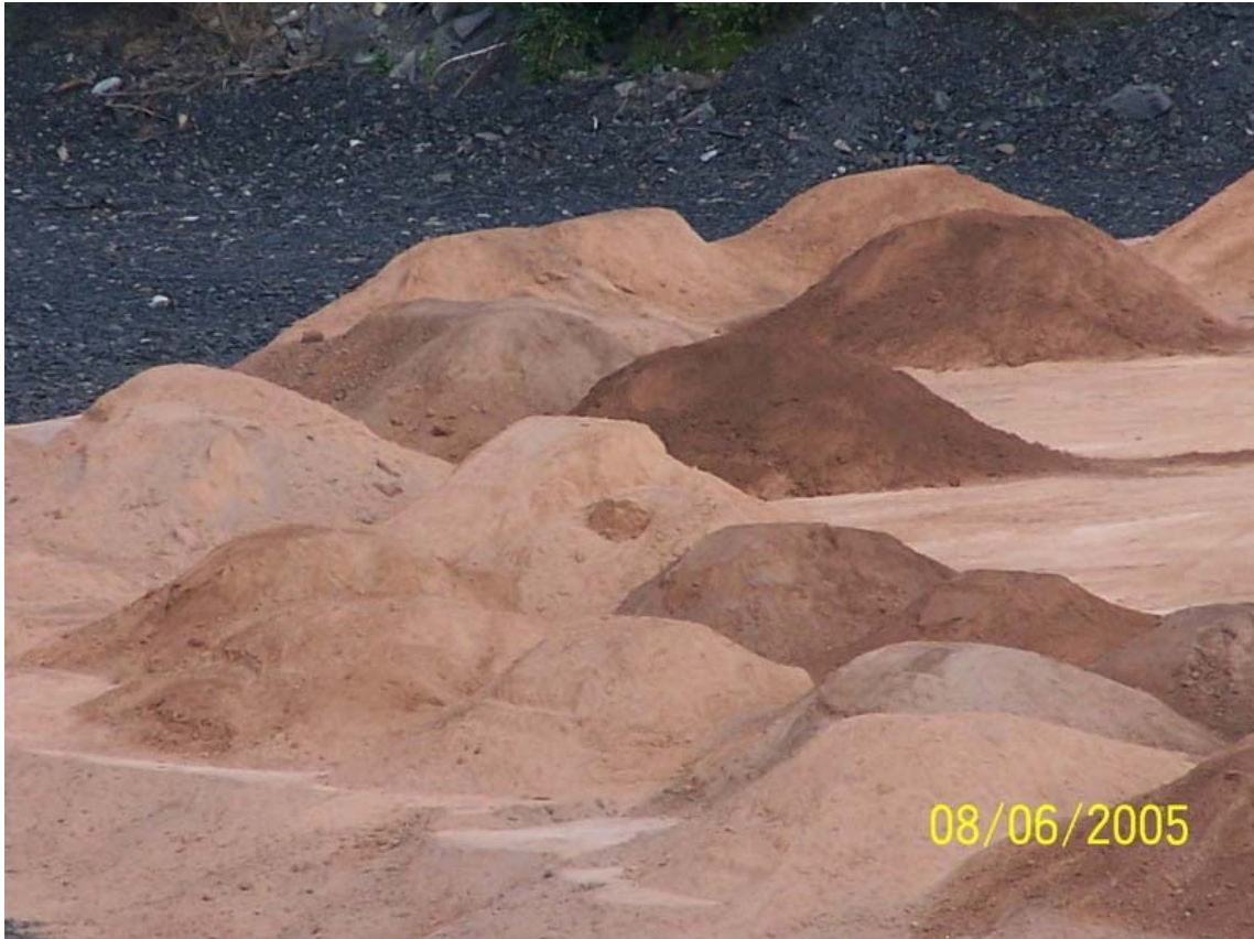
CAPTION - The reddish, tan, brown FBC waste coal ash placed in many Pennsylvania Mines stands out against darker gray and black coal refuse. Coal refuse and waste coal are one and the same and called “culm” if from anthracite coal or “gob” if from bituminous coal. Here FBC culm ash is being piled on top of culm and mine rock at the AC Fuels Co Mine in northern Schuylkill County, a site not examined in this report. Photo by Steven Dreyer, McAdoo, PA.
